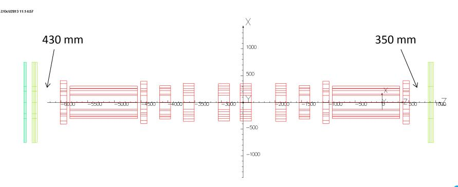
The position of the VP's assumes a gap to the coils of 390mm but the coils as implemented in the model (TRD) are shifted 40mm DS wrt this. I speculate that this has occurred because the US SS was pinned to its fixed location pre RFCC extensions.
