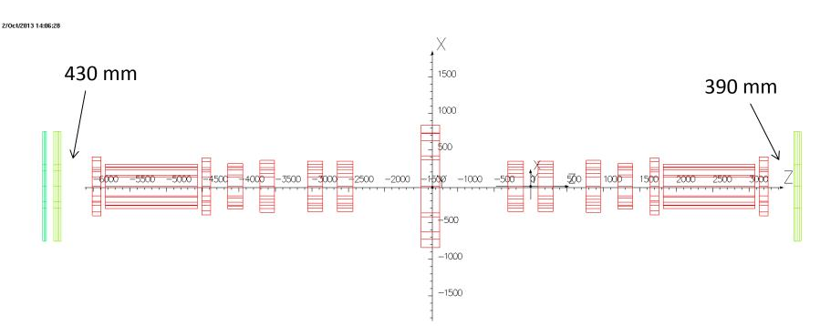
The position of the VP assumes a gap of 390mm but the coils are 40mm short of this at opera the US end because the TRD coils don't include the RFCC extensions. (This is 2x20mm per Coupling coil)
