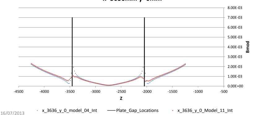
Comparison Plots of Field Behind Modelled Shield Wall at x=3636mm y=0mm
