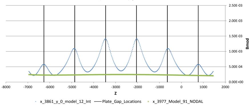
This is the same plot as from the earlier slide but I've added the nodal result from model 91 from behind the SSW. Not directly comparable as geometry is different for the SSW and SSW is slightly (116mm) further away from magnets but perhaps this gives a qualitative comparative indication of the effect of the gaps? 16/07/2013
