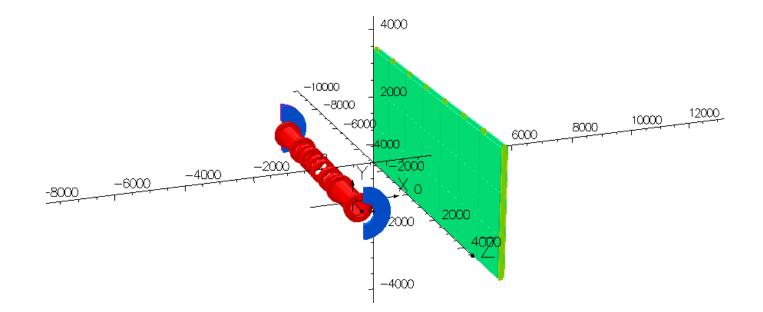
Shield Wall is 7 x 3 panels. 7mm gap between panels Panels are stood off from I beams by 1mm.
