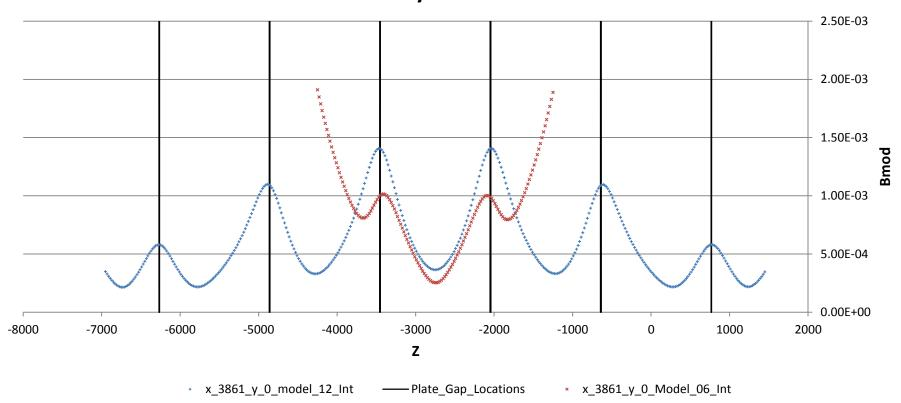
These are integral line plots. 3861mm represents approximately 10" behind the shield wall Model 06 is for the 2 x 3 plates and is with the plates in contact with the I beams. Model 12 is for the 7 x 3 plates and there is a 1mm gap between the plates and the I beams hence the larger field at the gaps. (The flux will find it harder to find a path through the I beam)
