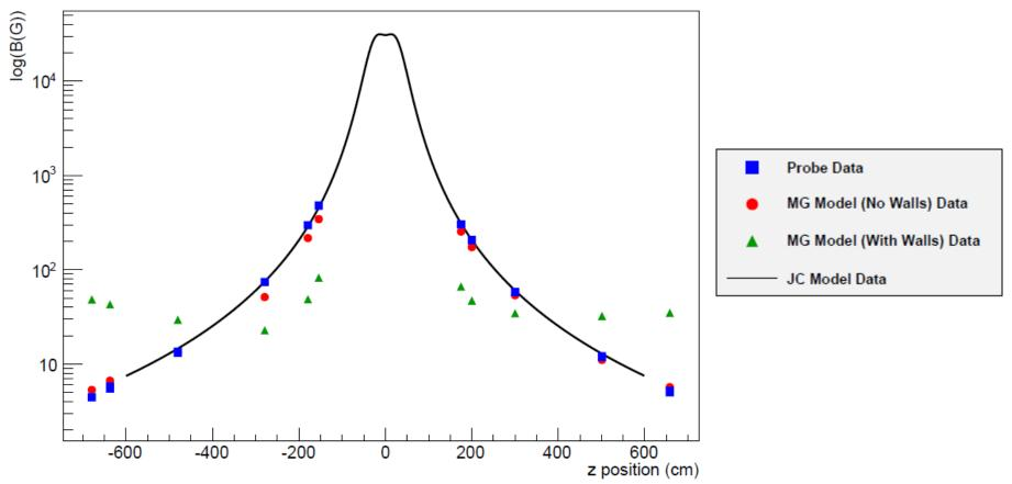
Blue points are measurements, red and green points are from Opera models, black line is Biot-Savart prediction.
