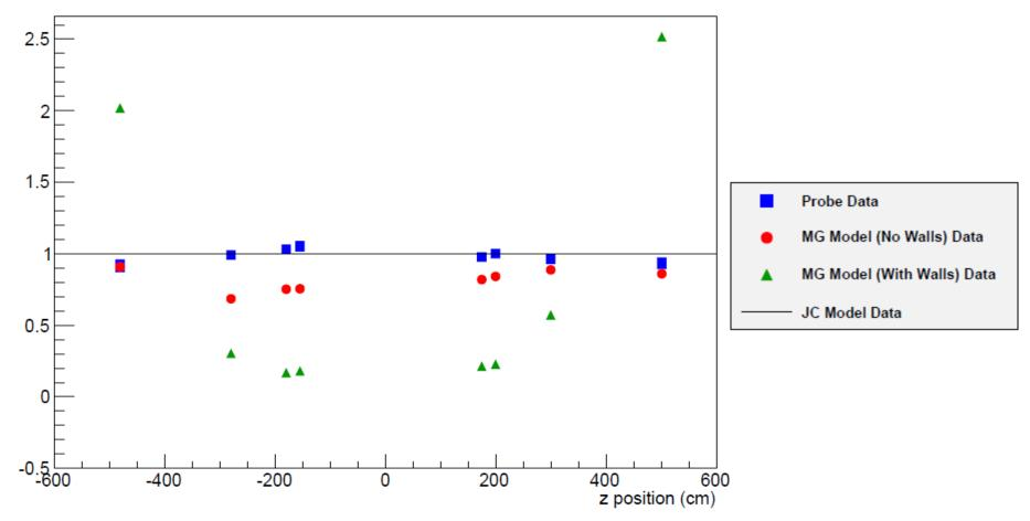
Blue points are measurements, red and green points are from Opera models, black line is Biot-Savart prediction. Model and probe data have been normalised to B-S prediction
