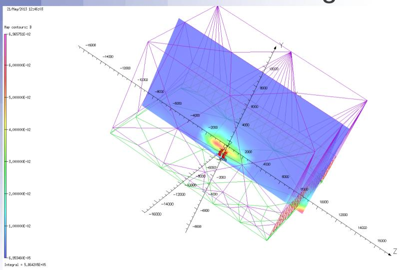
UNITS Length Magn Flux Density T Magnetic Field Magn Scalar Pot **Current Density** Power Force MODEL DATA R9ModelInc1010WallsV1.op3 **TOSCA Magnetostatic** Linear materials Simulation No 1 of 1 571092 elements 126778 nodes 2 conductors Nodally interpolated fields Activated in global coordinates **Field Point Local Coordinates** Local = Global FIELD EVALUATIONS Cartesian CARTESIAN (nodal) x=0.0 y=-600.0 to 9000.0
