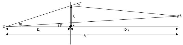
In this figure, the source S (white star) is lensed by L (whose centre is the black star) and observed at O. Note that for cosmological distances it is *not* in general true that  $D_{\rm S} = D_{\rm L} + D_{\rm LS}$ , despite the appearance in the diagram! We assume that the lens L can be approximated by a single object at a well-defined distance  $D_{\rm L}$ —the *thin lens approximation*—and that all the angles are small.
