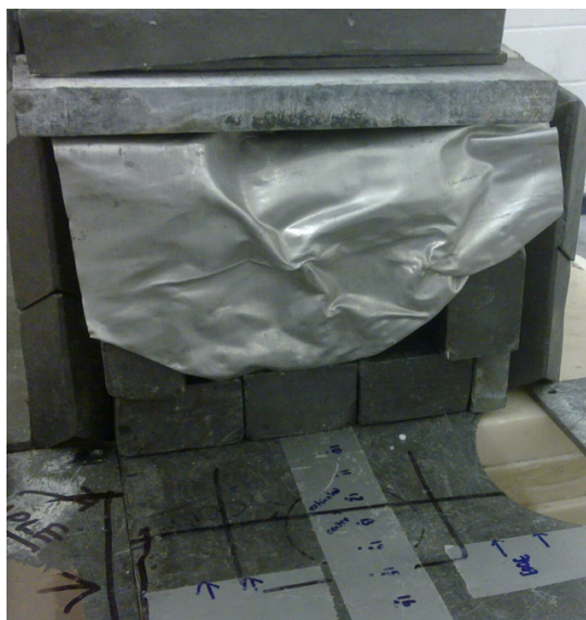
Figure 8.18: Cadmium foil wrapped around the NaI(Tl) crystal. The geometry of the lead shield and copper collar is unaltered.
