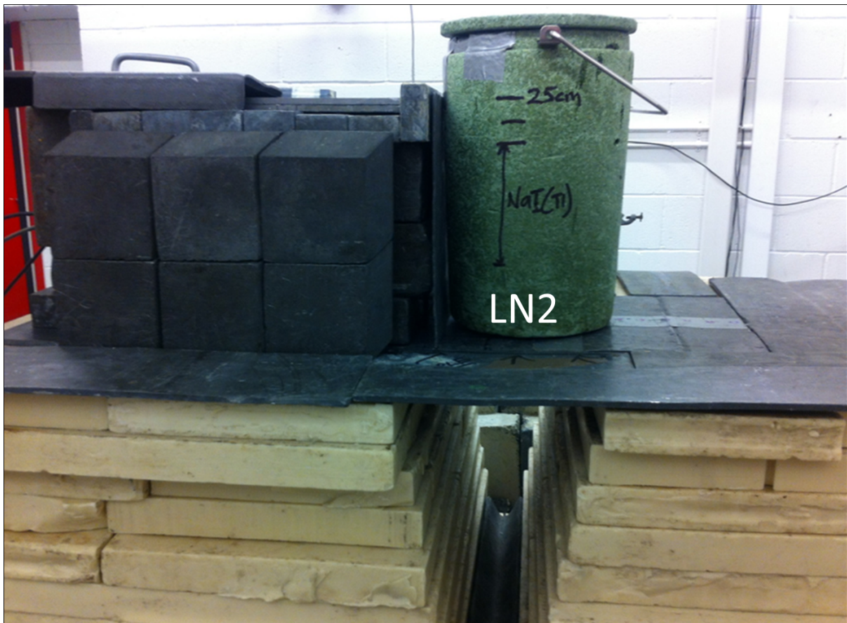
Figure 11.3: IMAGE OF LN2 DEWAR NEXT TO DETECTOR OVER APERTURE
