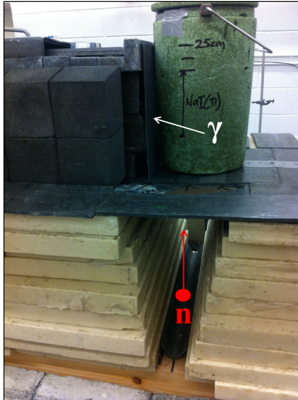
Figure 8.1: Figure showing the collimated neutron generator, shielded scintillation detector and sample location.
