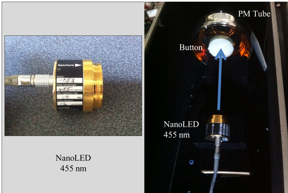
Figure 5.9: IBH NanoLED [18] system with a Hornyak style button coupled to a 5 inch diameter EMI 9791 KB photomultiplier tube
